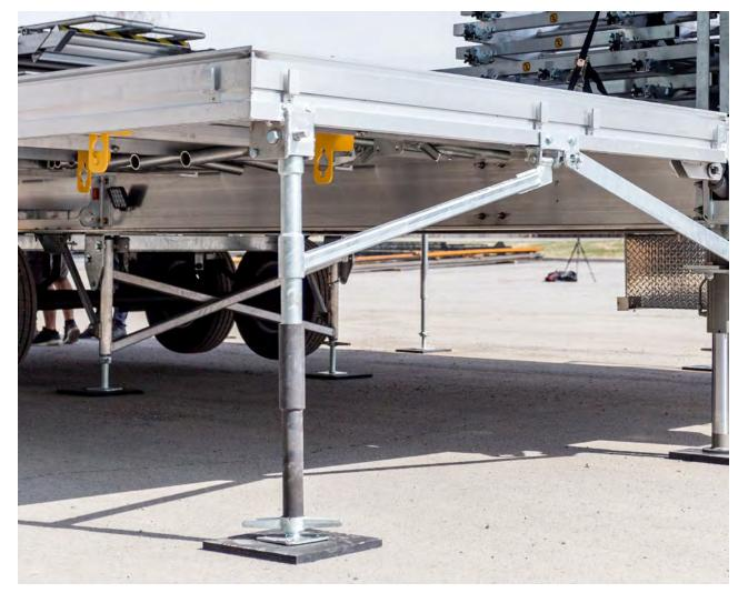
**Deck & chassis at 150 lb/ft²** (732 kg/m²) **meets IBC & NBC standards** Cross braced steel members added to support legs under the mid-section of trailer frame.
