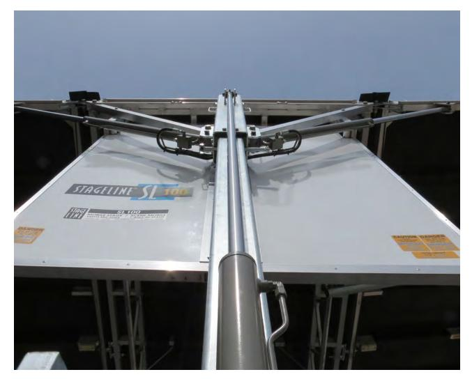
Raise & lower the roof securely with double mast lifting mechanism
