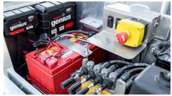
**Battery**Battery system for work lights, emergency breakaway system and engine starter.
